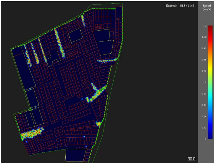
Fig. 14. Evacuation speed at 30 seconds before improvement. (Source: Authors, 2025)
