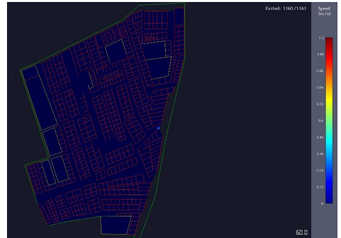
Fig. 17. Evacuation speed at 60 seconds after improvement. (Source: Authors, 2025)
