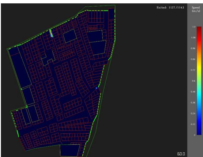
Fig. 16. Evacuation speed at 60 seconds before improvement. (Source: Authors, 2025)
