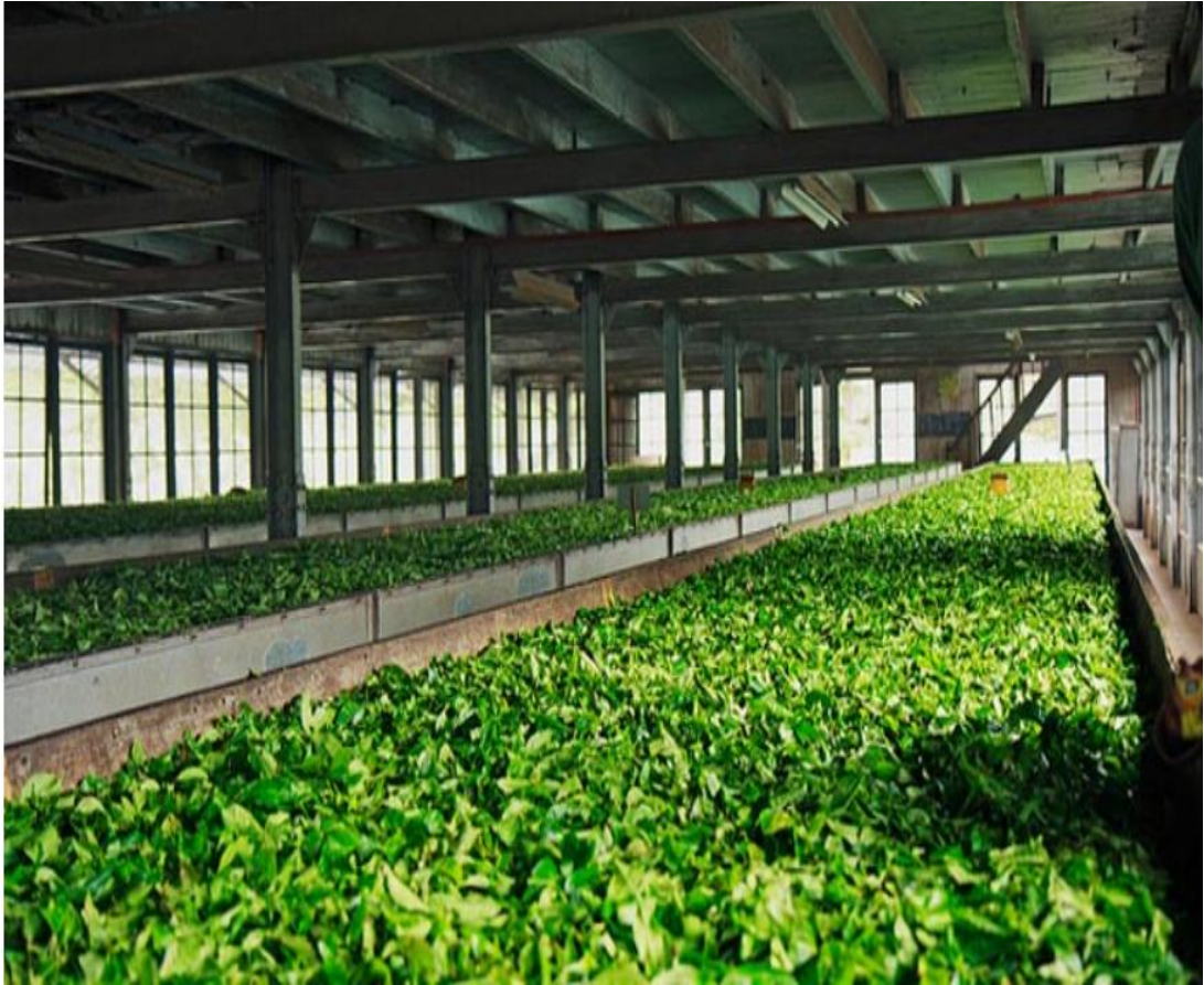
Figure 2. 2: Withering process (Deb & Jolvis Pou, 2016)
