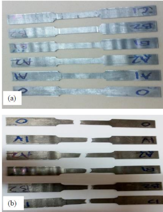
Figure 3.18: Tensile test samples (a) before fracture (b) after fracture
