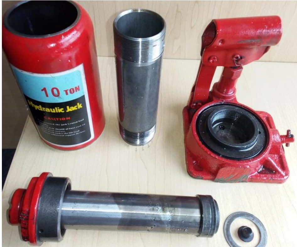
Figure 3.7: Parts of a dismantled jack
