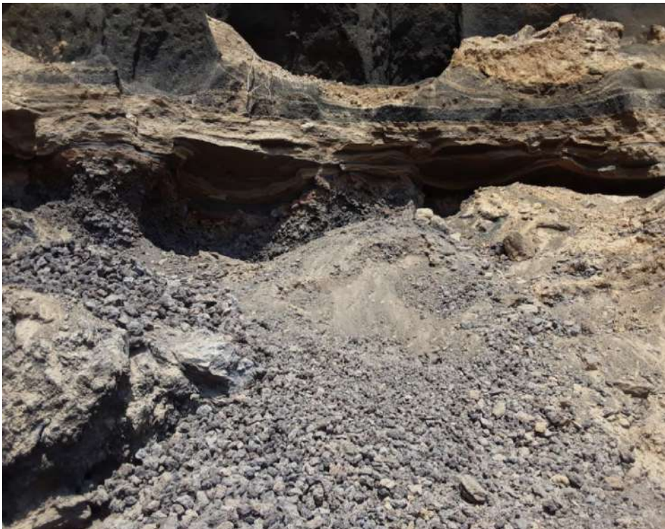
Figure 9: Photo of natural Cinder aggregates excavated at Ituha area.
