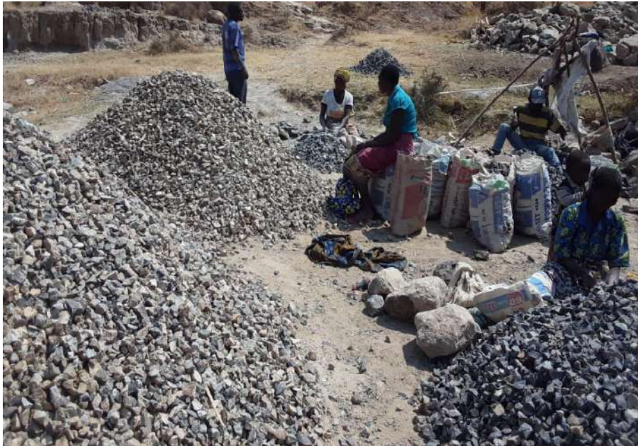
Figure 8: Photo of hand crushed aggregates from collected stones at Mbalizi area.
